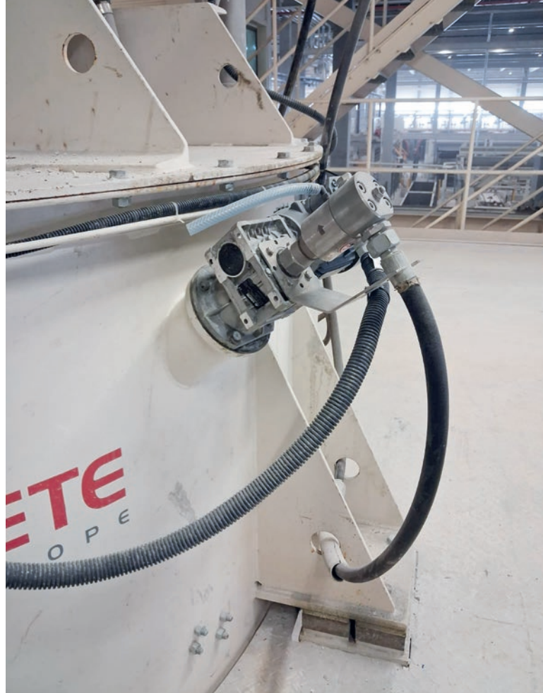
High-pressure cleaning nozzle installed on the AAC mixer.
