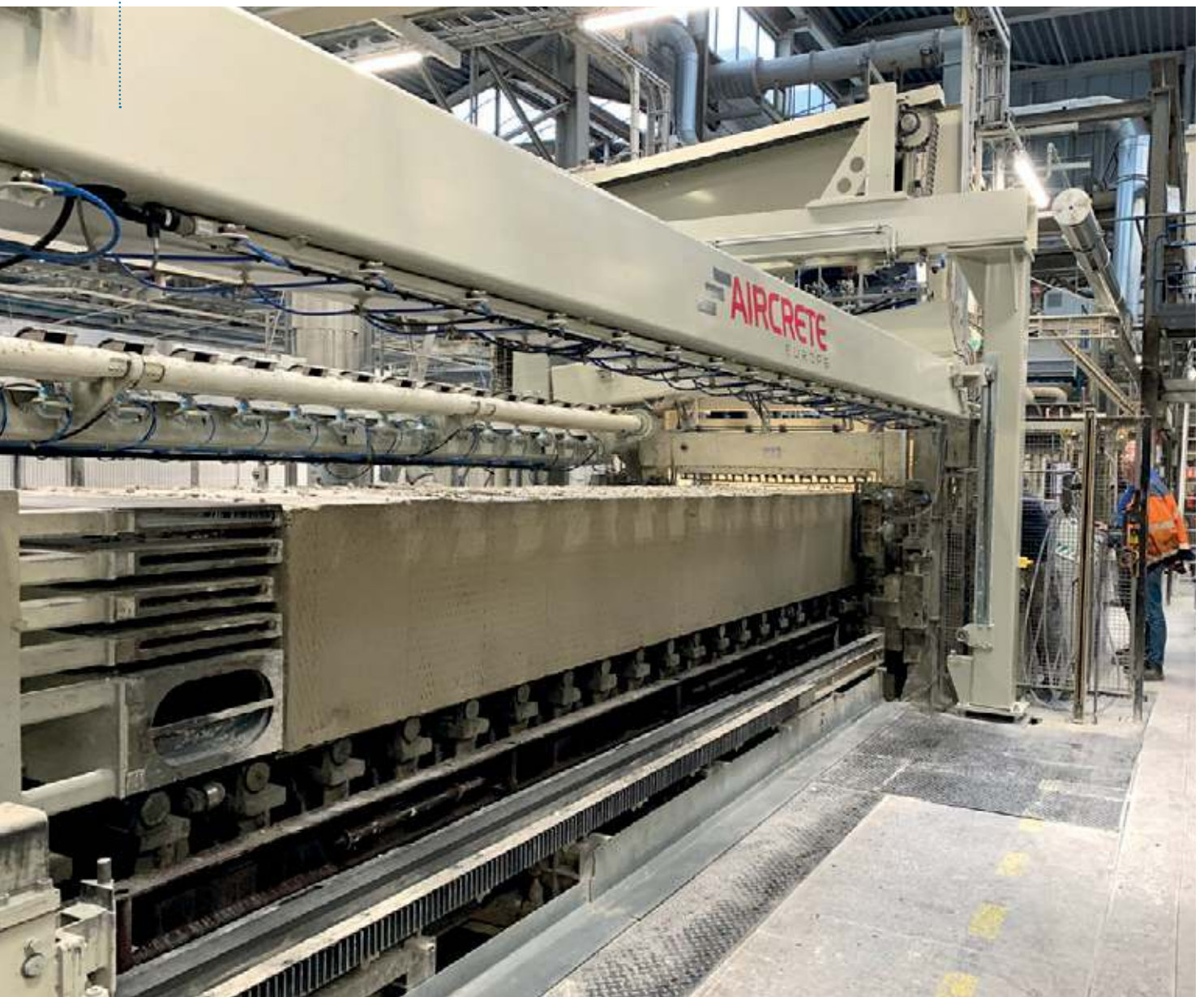
Fig. 1: Upgrade of the first section of Xella Vuren's cutting line with the replacement: Aircrete Cross Cutter.
