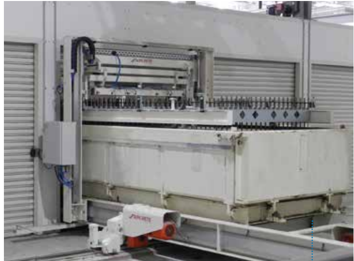
Fig. 8: The automatic unlocking system detaches the needles from reinforcement inside the cake after pre-curing
