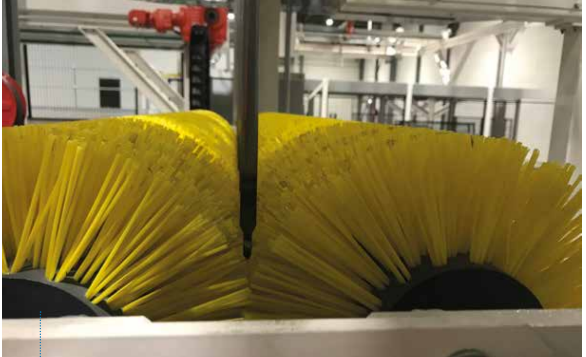
Fig. 9: The automatic needle brushing unit cleans the slurry residue on the needles
