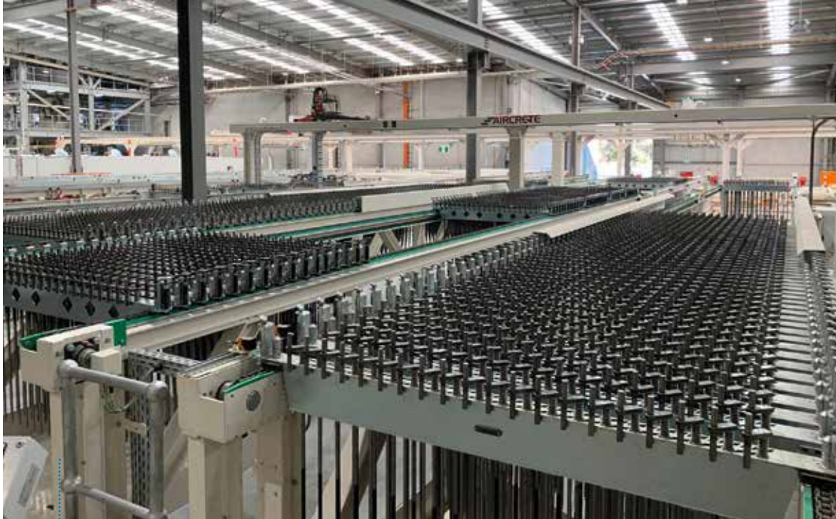
Fig. 4: A magazine of cross bars from which the correct reinforcement frame is configured as per the batch request from the MES
