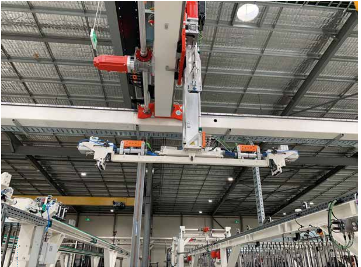
Fig. 5: The multi-axis robot that selects the right cross bar with the right needles
