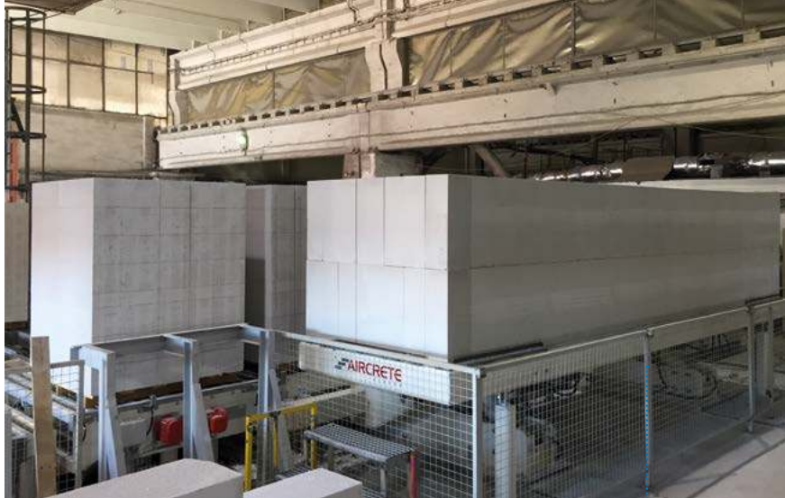
Fig. 4: The pallets are transported to the foiling machine one by one automatically
