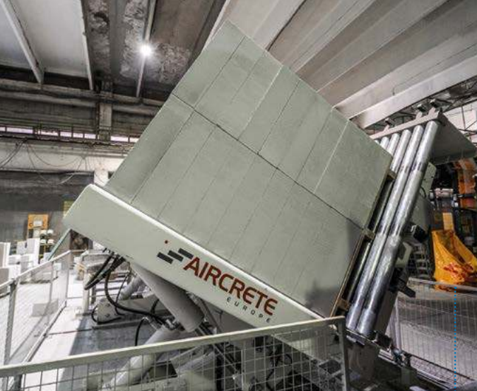
Fig. 3: The blocks are tilted 90° in order to stack them on the pallets on their larger surfaces
