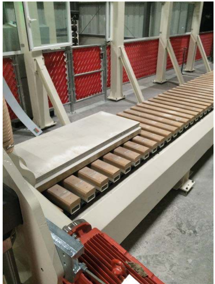
Fig. 9 and Fig. 10: The infeed and outfeed of the sawing line with the dust vacuum suction unit at Aircrete Mexico plant that profiles on the sides of the panels
