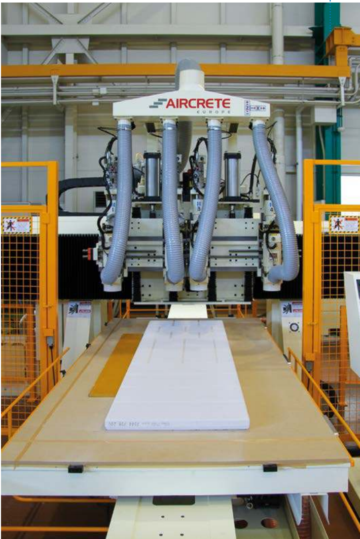
Fig. 6: Aircrete panel milling system can mill two panels at once
