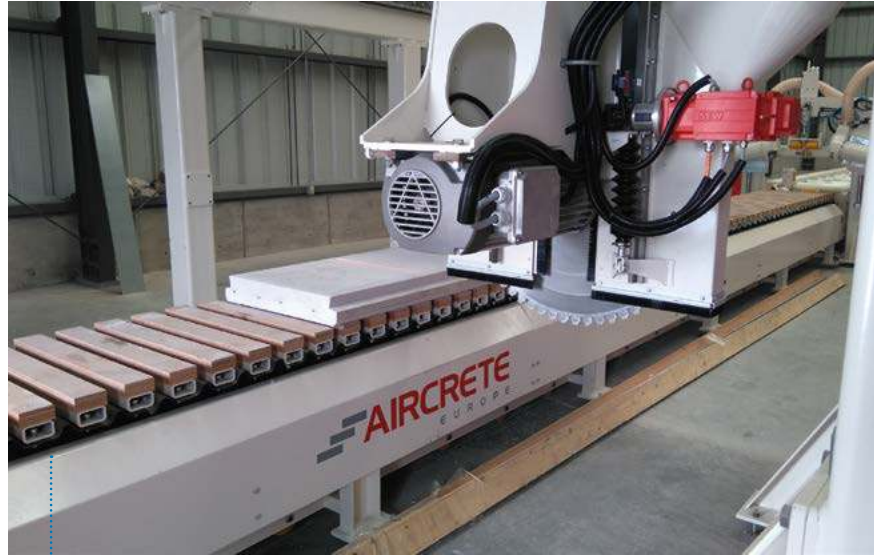
Fig. 8: With the head that can move up to 90°, the sawing machine at Aircrete Mexico cuts the panels in the desired shape
