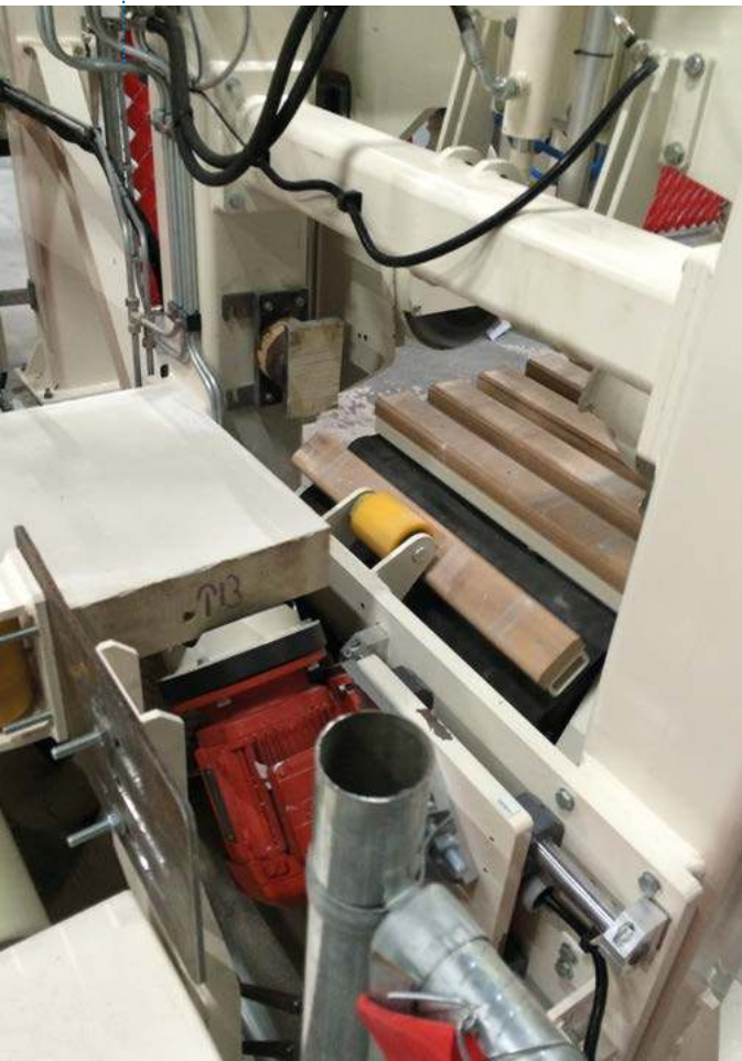
Fig. 9 and Fig. 10: The infeed and outfeed of the sawing line with the dust vacuum suction unit at Aircrete Mexico plant that profiles on the sides of the panels
