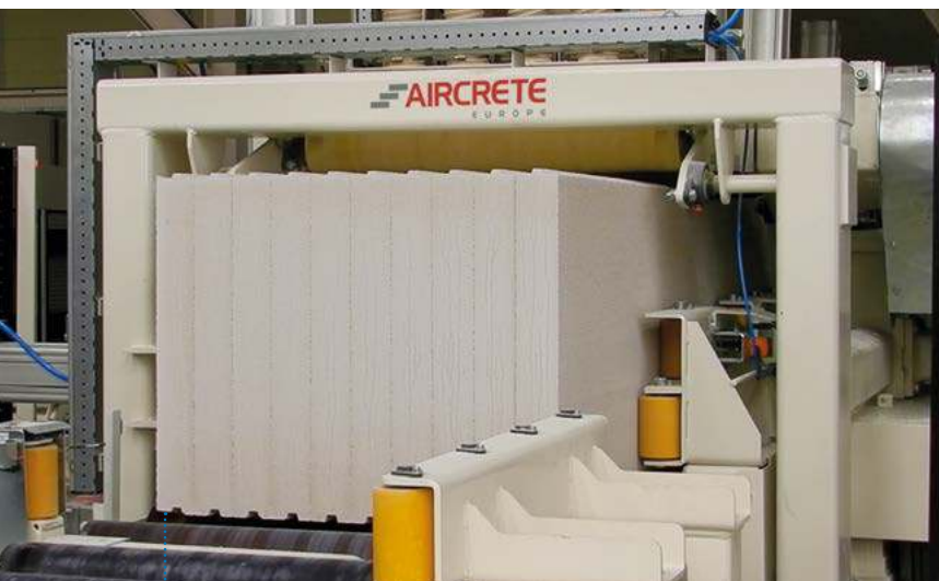
Fig. 2: Fully profiled panels exiting the milling unit
