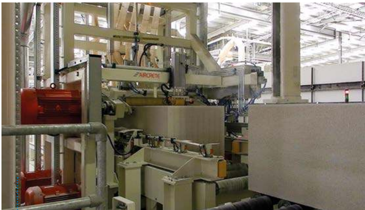
Fig. 1: Panels as they feed into the panel pack milling unit
