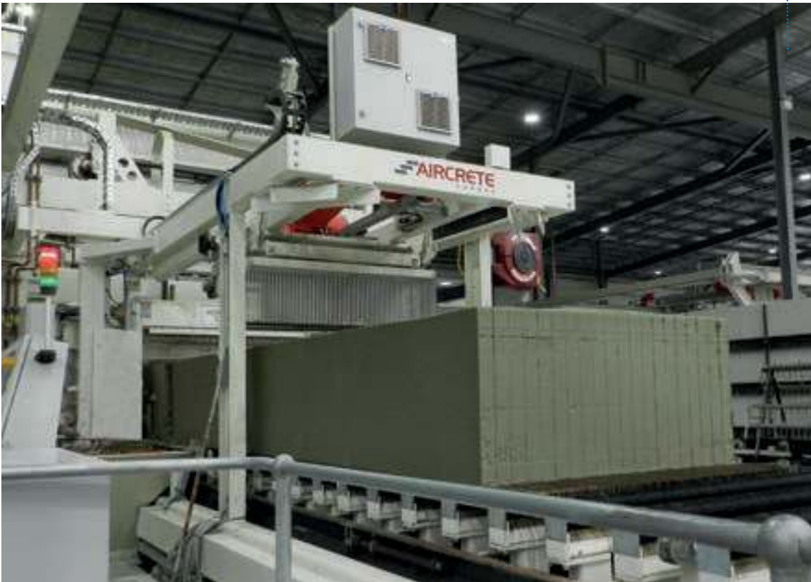
Fig. 4: After the completion of the project, Aercon will be the first factory in the US with the Aircrete flat-cake cutting line
