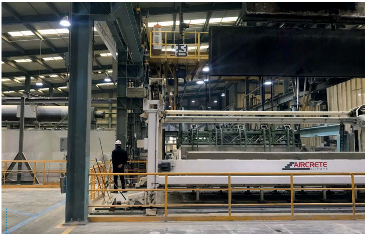
Fig. 1: Aircrete Europe was also engaged as SYC's technology partner in 2013 for the upgrade project from a Hebel to a Durox flat-cake cutting system.
