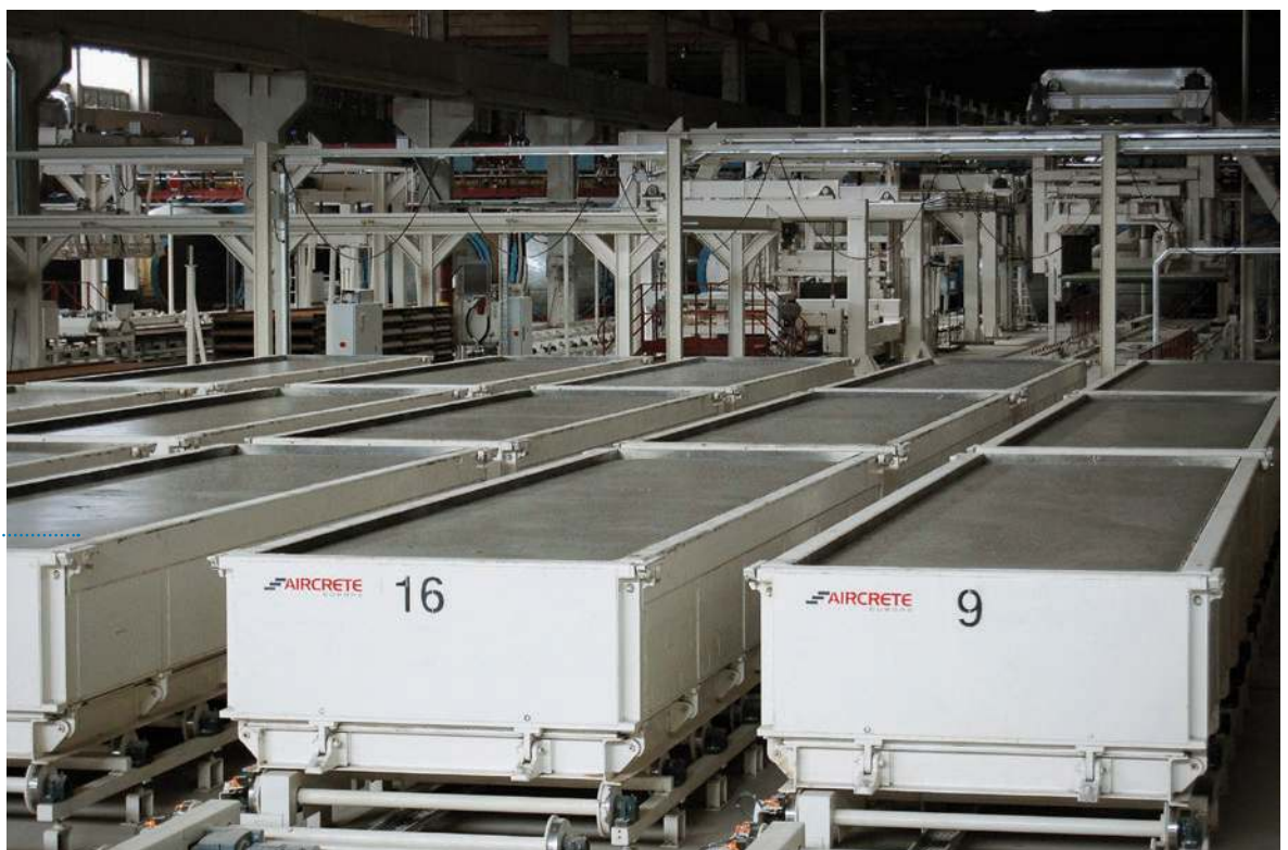
Fig. 7: All the moulds within the Aircrete Europe plant are adjustable in length and they carry configuration information for each product type and are traced individually.
