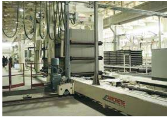
Fig. 10 A traverser car transfers the triple stacks to the autoclave.
