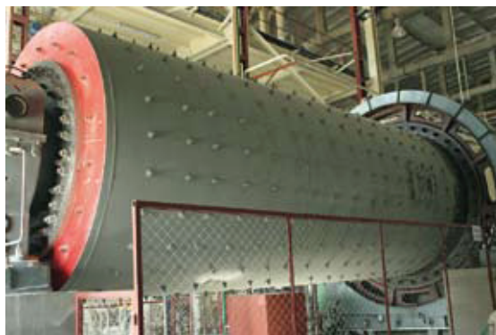
Fig. 1 The ball mill is used to reduce the size of the sand particles to powder. The sand and water are grinded to a fresh slurry.
