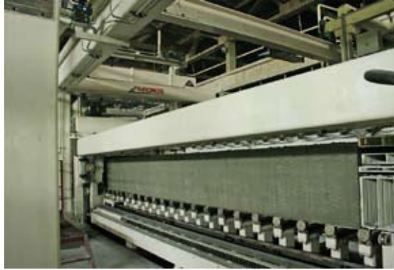
Fig. 7 Aircrete's cutting machine with high-speed moving dual-wire cutting frames.
