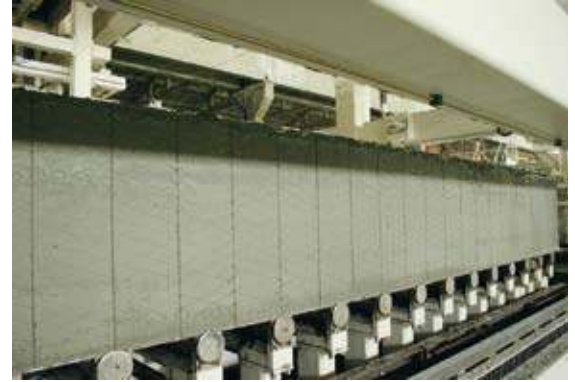
Fig. 8 The cross-cutting frame cuts the blocks to height by dragging the wires through the cake.
