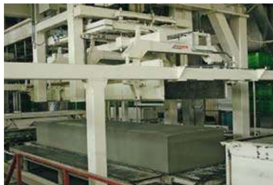
Fig. 6 The grabbing crane picks up the flat "green" cake for transport to the cutting machine.
