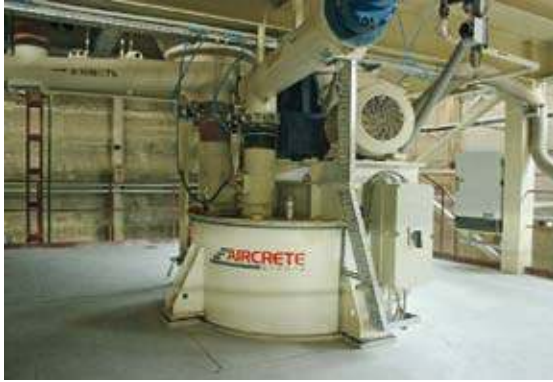
Fig. 3 Computer-based mixing control system for mixing and dosing of the raw materials.
