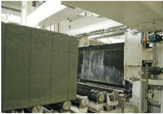
Fig. 9 The horizontal and vertical cutter cut the blocks to length and thickness.
