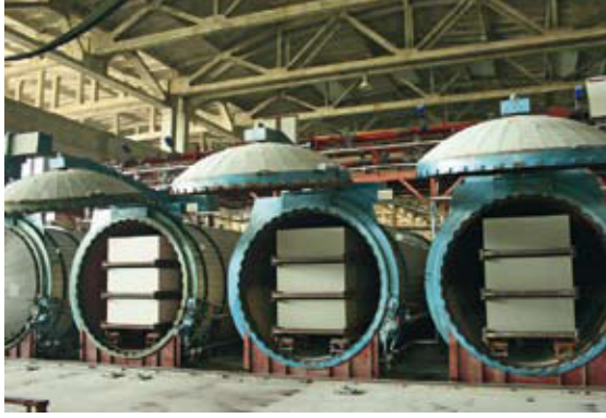
Fig. 11 Cakes are cured in the autoclaves at a steam pressure of approximately 12 bar. A complete autoclave cycle is between 12 and 15 hours long.
