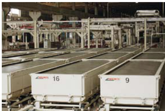
Fig. 5 A transfer car moves the molds to the swelling area.
