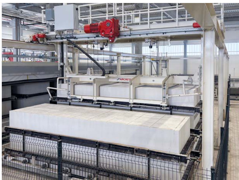
Fig. 8: Stacking/De-stacking Manipulator that provides flexible pack configurations for efficient downstream packaging and dispatch.
