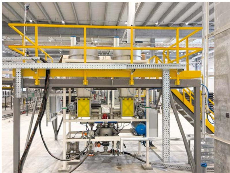
Fig. 3: New Aircrete Batch-by-Batch Aluminium System.
